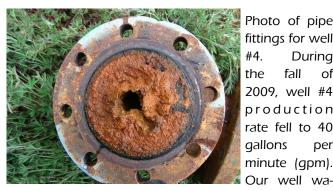
ter production goal is 200 gpm per well. The pipe opening is 6-inches in diameter and has been reduced to 1-inch in diameter from the iron deposits. The iron deposits are removed before reassembly of the fittings and placing the well back into service.
