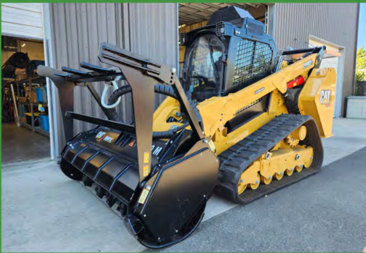
CAT 299D Compact Track Loader with mulcher attachment
