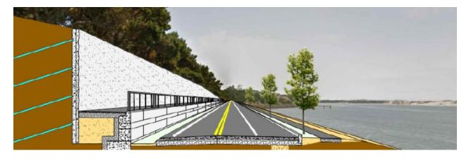
One of the key features of the project is dealing with the slopes on the east side of Rhododendron Drive south of New Hope Lane. The project utilizes the slope to the benefit of the project by incorporating the multi-use path and elevating it in this section of the project. This will allow pedestrians and bicyclists a view of the river and sand dunes from above motor vehicle level.
