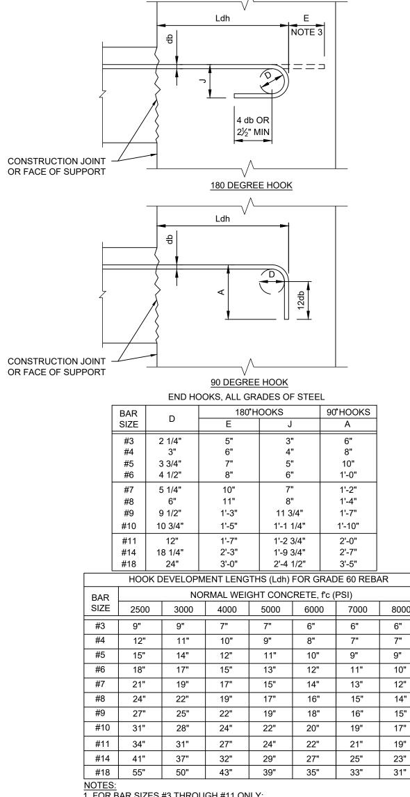
NOTES: 1. FOR BAR SIZES #3 THROUGH #11 ONLY: a. IF CONCRETE SIDE COVER IS ≥ 2½" AND END COVER ≥ 2", THEN A MODIFICATION FACTOR OF 0.7 MAY BE APPLIED BUT THE LENGTH MUST NOT BE LESS THAN 8 BAR DIAMETERS NOR 6 IN. 2. FOR EPOXY-COATED HOOKS, MULTIPLY THE TABULATED VALUES BY 1.2. 3. BAR DIMENSION REQUIRED TO MANUFACTURE HOOK 3 STANDARD HOOKS AND EMBEDMENT 1 1/2" = 1'-0"
