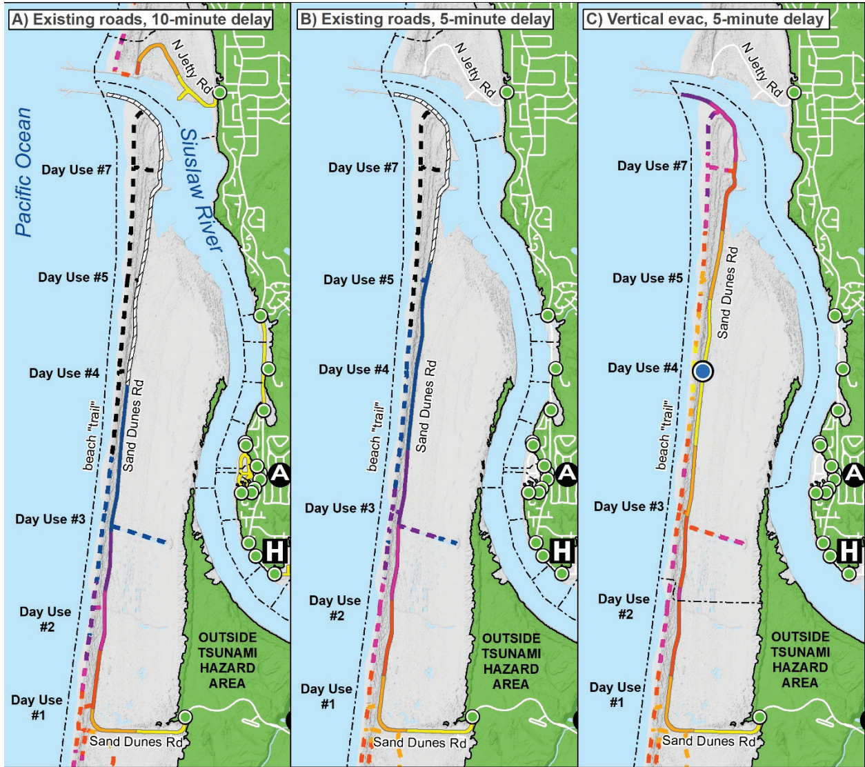
Figure 3-18. Beat the wave minimum walking speeds for the South Jetty Area. A) assuming the existing road network remains intact, B) reducing the evacuation delay to 5-minutes, and C) a hypothetical vertical evacuation structure at Day Use #4. Black dashed lines indicate trails 'unlikely to survive (>10 mph).
