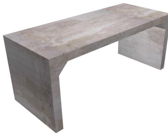
Figure 6-23 - Section of pre-cast concrete box culvert
