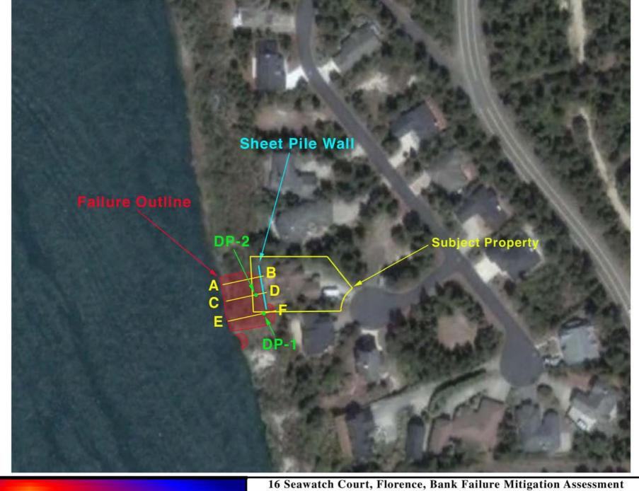
Figure 3: Failure, Field-developed Cross Section and WRDP Locations
