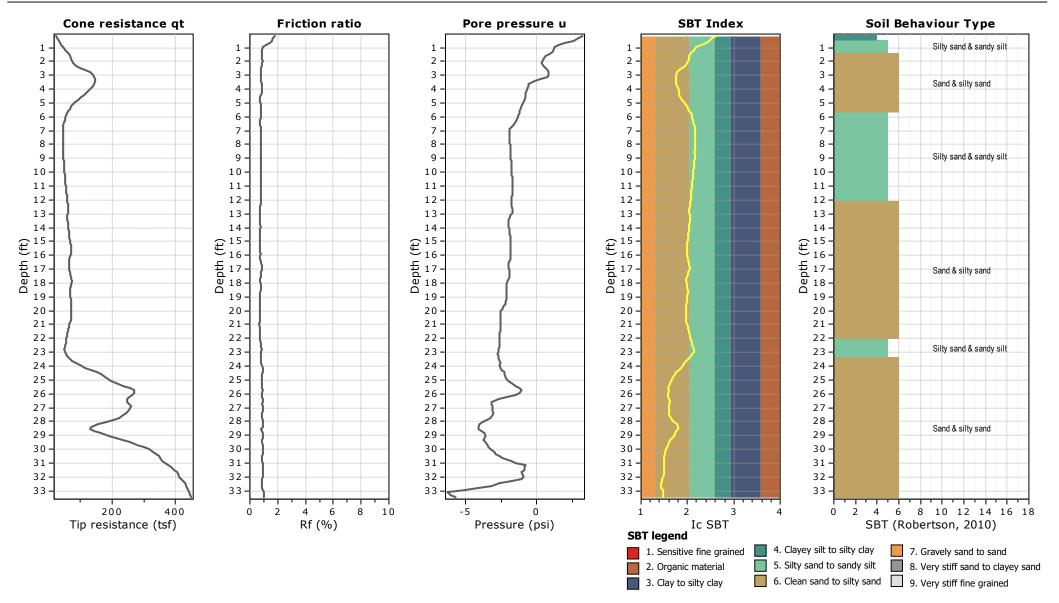
Total depth: 33.47 ft, Date: 2/23/2021 Surface Elevation: 47.00 ft Coords: X:43.97, Y:-124.10 Cone Type: Vertek Cone Operator: Oregon Geotechnical Explorations
