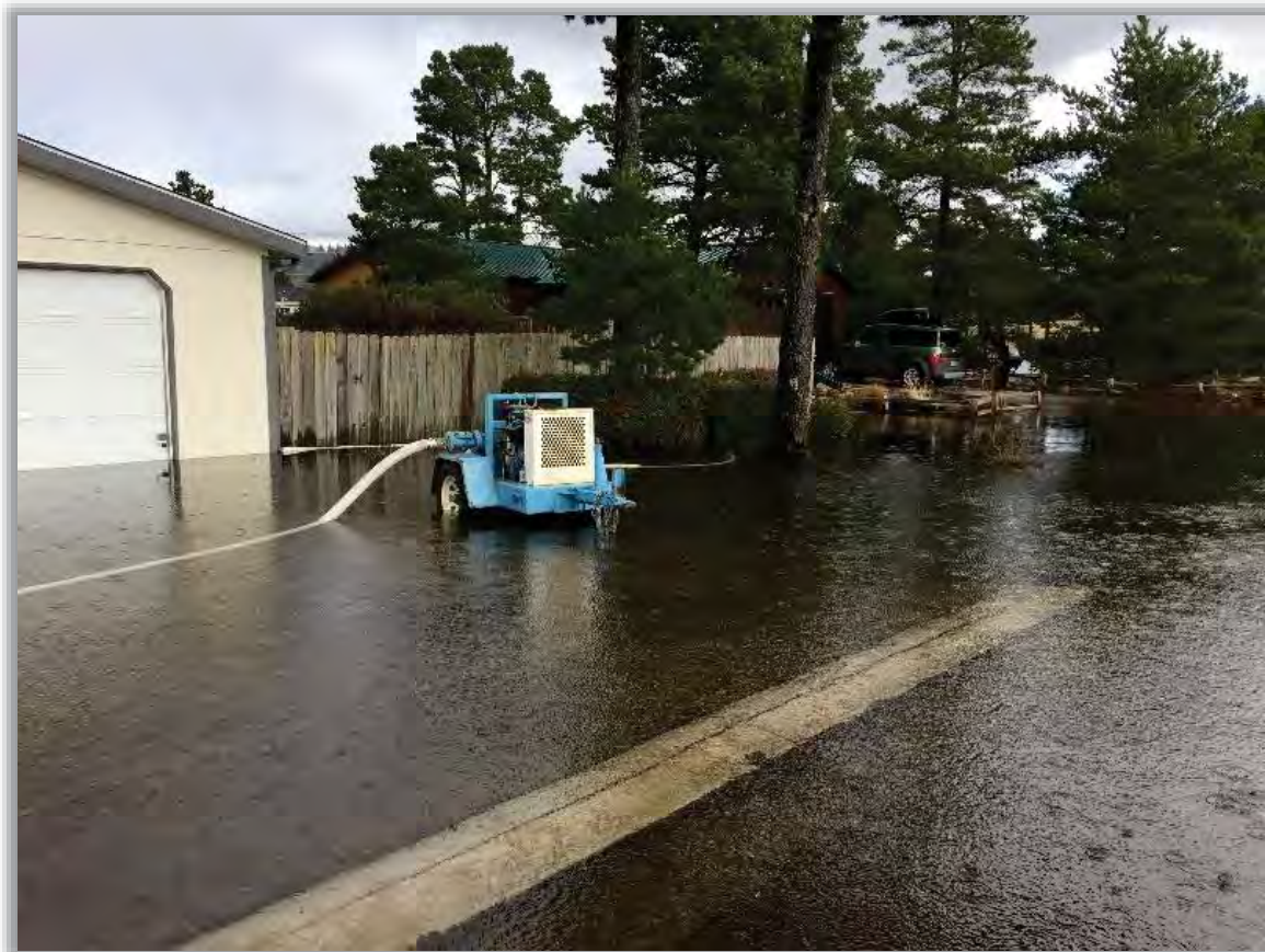
Figure 4-45 - Driveway of 1720 Pine Court, pumping flood waters west across Willow Loop into Munsel Creek
