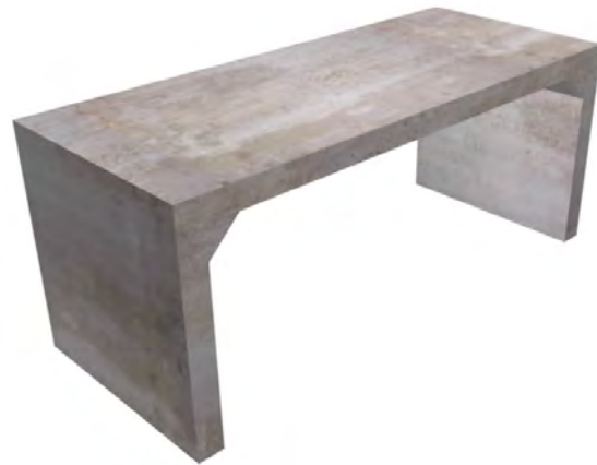
Figure 6-23 - Section of pre-cast concrete box culvert
