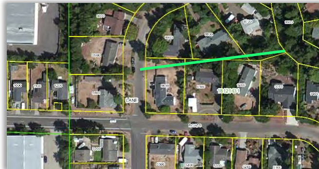
Figure 6-2 - Tax lots near 42nd and Spruce. Direct discharge into Munsel Creek would require easements
