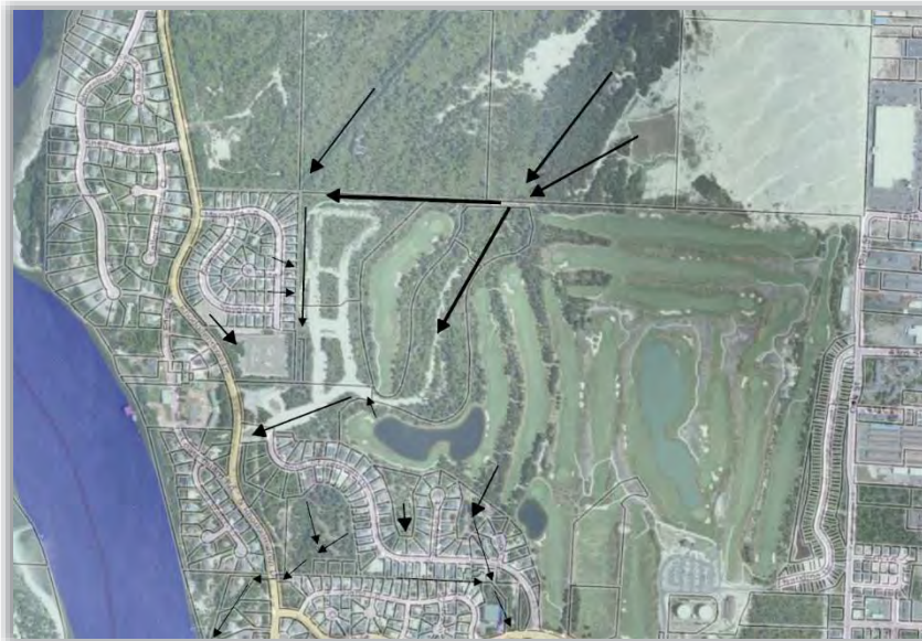
Figure 4-12 - Surface & ground water movement near Mariner's Village
