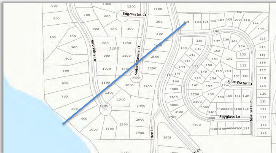
Figure 6-9 - Mariner's Village vicinity map, showing possible path of directionally bored pipe from Tax Lot #300 to the Siuslaw River
