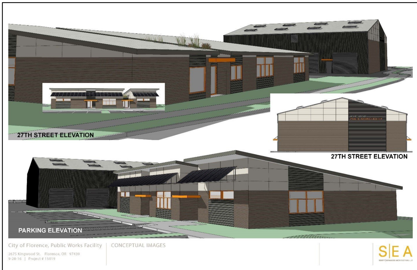
Public Works Operations Facility architectural renderings show the plans for the future office and maintenance buildings.
