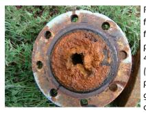
Photo of pipe fittings for well #1. During the fall of 2010, well #1 production rate fell to 40 gallons per minute (qpm). Our well water production goal is 200 apm per well. The pipe opening is 4-inches in
